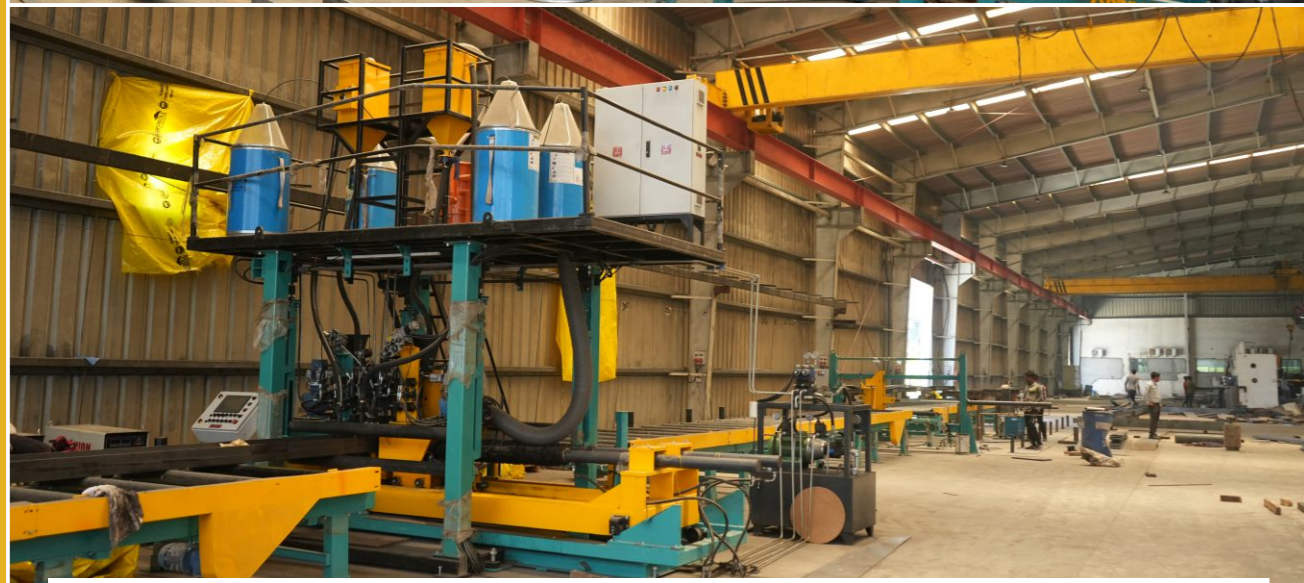
Line-2 PHI & Assembly with automatic welding machine (SAW).
