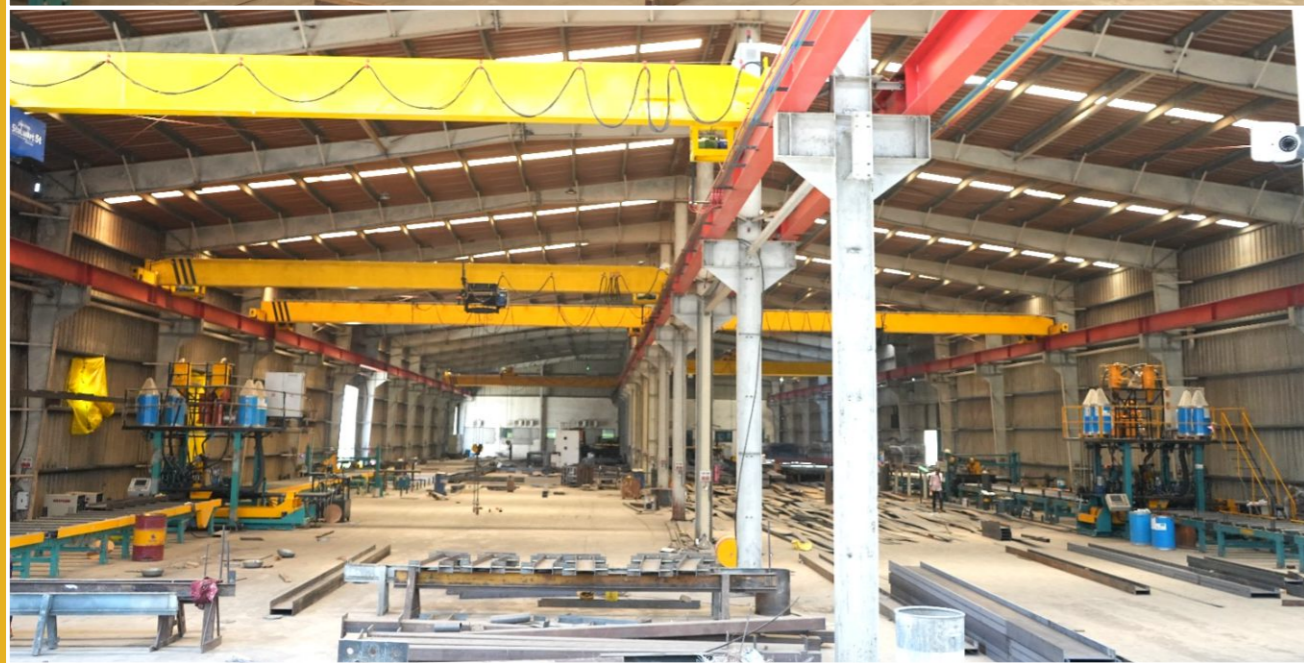
Line-2 PHI & Assembly with automatic welding machine (SAW).
